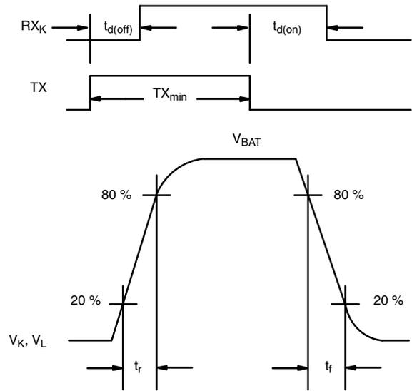
$R_L = 510 \Omega$ ,  $C_L = 10 \text{ nF}$ ,  $V_{BAT} = 6 \text{ V to } 18 \text{ V}$
