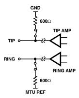
FIGURE 2. LPS 2-WIRE INTERFACE CIRCUIT DIAGRAM
