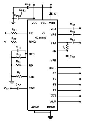
FIGURE 14. HC55183 BASIC APPLICATION CIRCUIT
