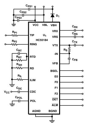
FIGURE 15. HC55184 BASIC APPLICATION CIRCUIT
