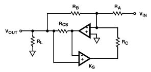
FIGURE 3. VOLTAGE FEED CURRENT SENSE DIAGRAM
