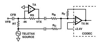
FIGURE 18. TELETAX SIGNALLING
