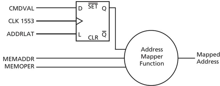
Figure 6 • Memory Address Mapping
