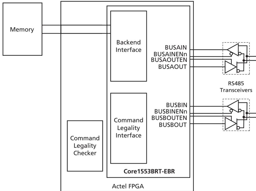
Figure 9 • Typical CPU and Memory-Based RT System
