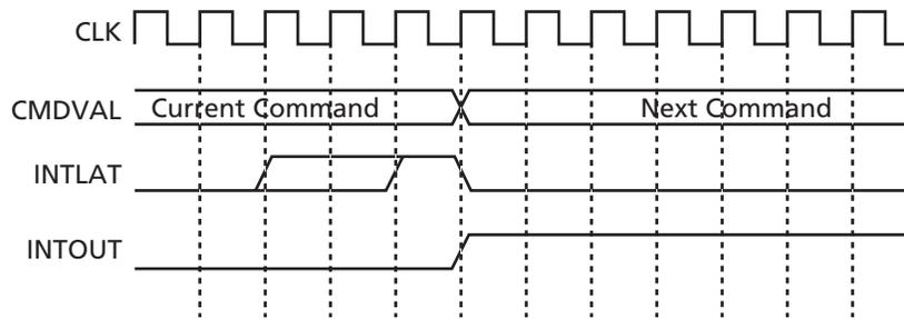
**Note:** This figure shows worst-case timing when a second 1553EBR command arrives as the core asserts an interrupt request. Also, INTLAT may be active for several clock cycles prior to INTOUT.
