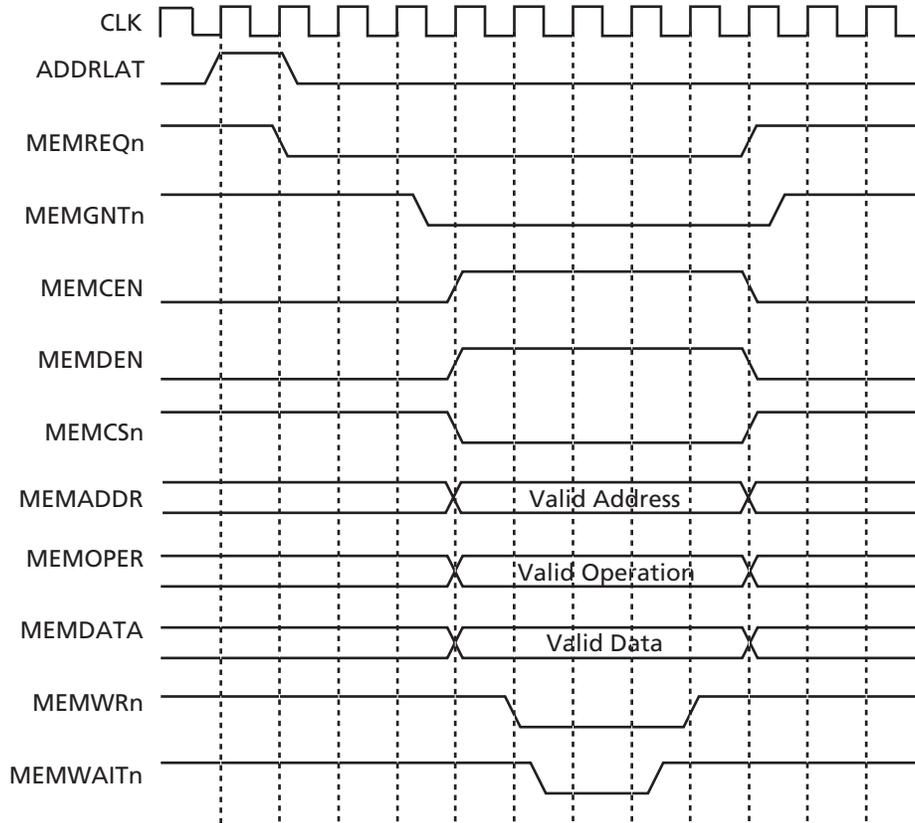
Figure 11 • Memory Write Timing – Asynchronous Mode
