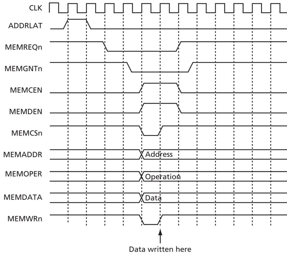
Figure 13 • Memory Write Timing – Synchronous Mode
