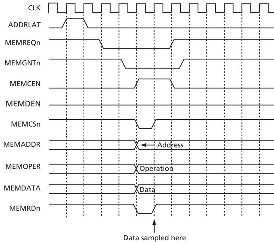
Figure 14 • Memory Read Timing – Synchronous Mode
