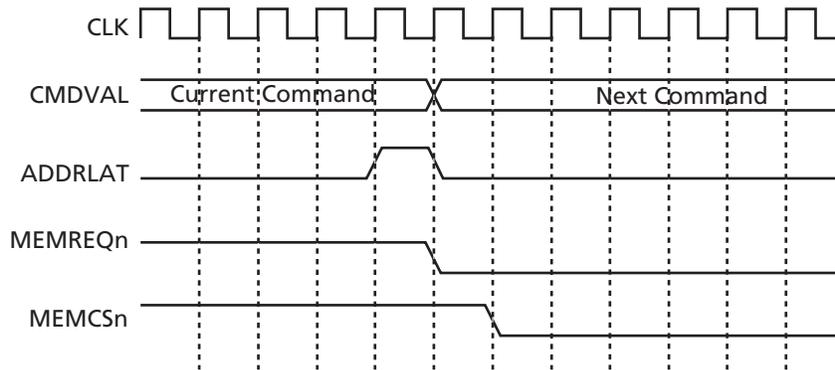
**Note:** This figure shows worst-case timing when a second 1553EBR command arrives as the core starts a backend transfer and MEMGNTn is held low.
