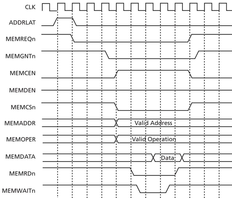
Figure 12 • Memory Read Timing – Asynchronous Mode
