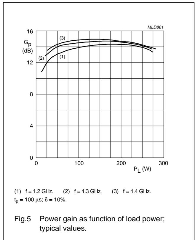
L-band radar LDMOS transistor
