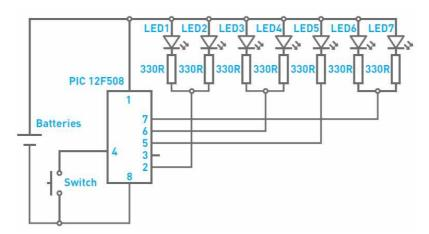
At the heart of the electronic circuit is a PIC microcontroller. A microcontroller is, in effect, a small computer. The circuit uses a push switch to detect when it should start generating the next number to be displayed. When the button is pressed the PIC very rapidly cycles through number 1 to 6, upon release of the button the number is displayed. The PIC then determines which of the LEDs should be lit up and sets pins 2, 5, 6 and 7 as required.
