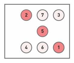
So, for example, if the number 3 (shown right) was to be displayed on the dice, this would require LEDs 1, 2 and 5 to be lit. These are controlled by PIC pins 2 and 5 (pin 2 controls LEDs 1 and 2). As the cathode of the LEDs are permanently connected to V+, the LEDs are turned on by taking their associated PIC pin low. This creates a voltage across the LED(s) and turns it/them on.
