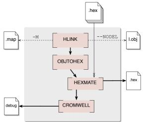
Figure 2.2: Flow diagram of the final compilation sequence
