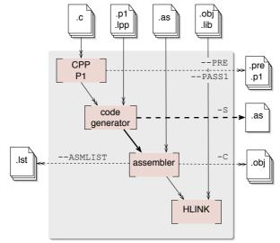
Figure 2.1: Flow diagram of the initial compilation sequence
