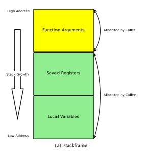
Figure 3.1: General Function Stack Frame
