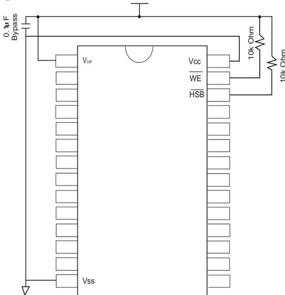
If the power supply drops faster than 20 us/volt before  $V_{CC}$  reaches  $V_{SWITCH}$ , then a 2.2 ohm resistor should be connected between  $V_{CC}$  and the system supply to avoid momentary excess of current between  $V_{CC}$  and  $V_{CAP}$ .
