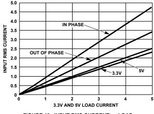
FIGURE 19. INPUT RMS CURRENT vs LOAD
