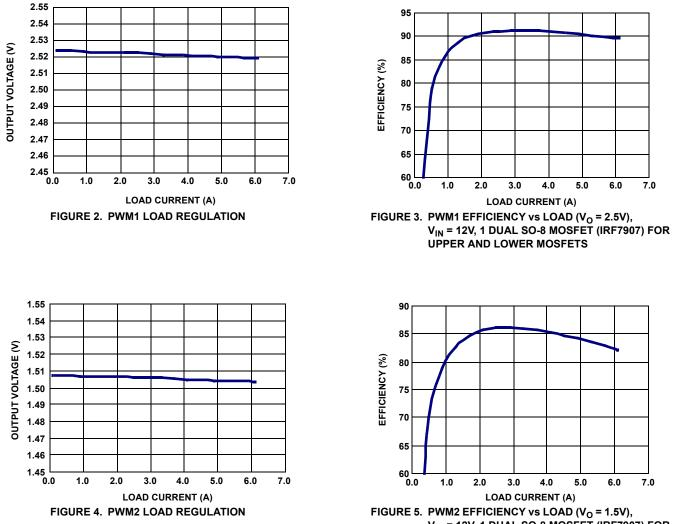
V<sub>IN</sub> = 12V, 1 DUAL SO-8 MOSFET (IRF7907) FOR UPPER AND LOWER MOSFETS
