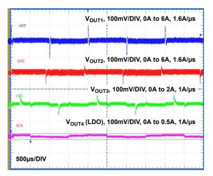
FIGURE 13. OUTPUT RIPPLE UNDER TRANSIENT LOAD
