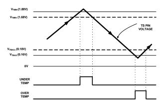
FIGURE 1. THRESHOLD VOLTAGES FOR 0°C to +50°C **WINDOW**
