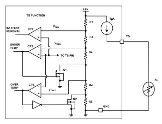
FIGURE 2. INTERNAL CIRCUIT FOR NTC INTERFACE
