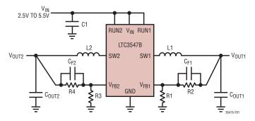
Figure 1. LTC3547B General Schematic
