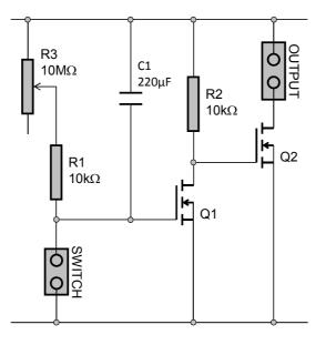
The circuit is triggered when the switch is pressed. At this point, current flows through the switch and charges the capacitor C1. When the switch is released the capacitor will still be full of charge and starts to discharge through R1 / R3. As the capacitor discharges there is less and less voltage across it, as this happens the voltage on the gate of the FET (Q1) gets closer to the positive voltage of the circuit.
