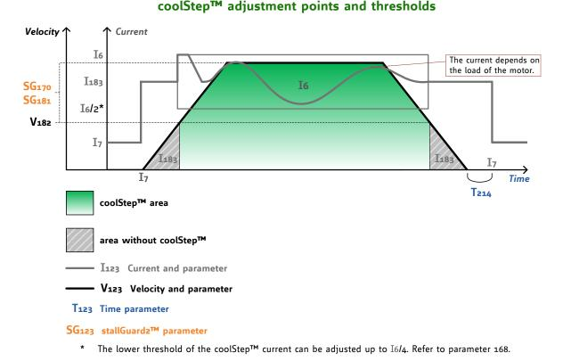
Figure 4.1: coolStep™ adjustment points and thresholds
