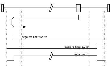
Search home switch in negative direction, reverse the direction when left stop switch reached.
