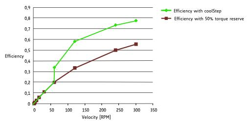
Figure 1.2 Energy efficiency example with coolStep
