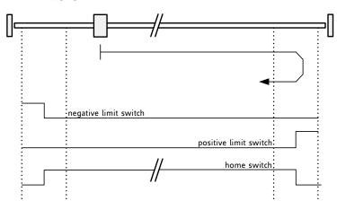
Search home switch in positive direction, reverse the direction when right stop switch reached.
