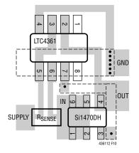
Figure 10. Layout for N-Channel MOSFET Configuration
