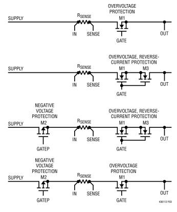
Figure 3. MOSFET Configurations
