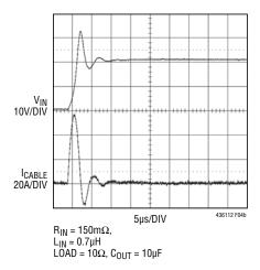
Figure 4. 20V Hot-Plug into a 10µF Capacitor
