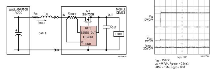
Figure 5. 20V Hot-Plug into the LTC4361
