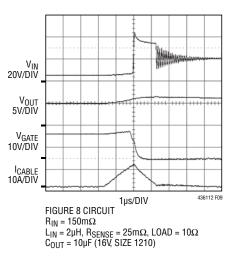
Figure 9. Overvoltage Protection Waveforms When 20V Plugged into 5V System
