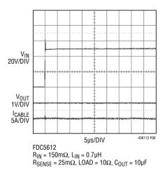
Figure 6. 50V Hot-Plug into the LTC4361
