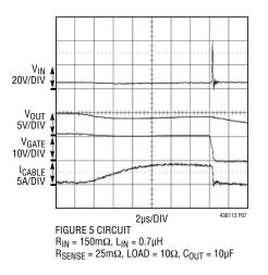
Figure 7. Overcurrent Turn-Off and Resulting Input Transient
