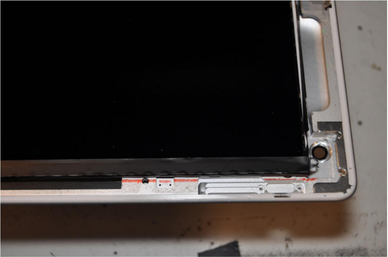
For the corner on the same side, but closer to the dock connector, a small section must be ground down. You should not cut this piece completely off, as it will be good to have support underneath the Retina Display's mounting bracket. You should shave a millimeter or two down. The area is marked with orange marker here.
