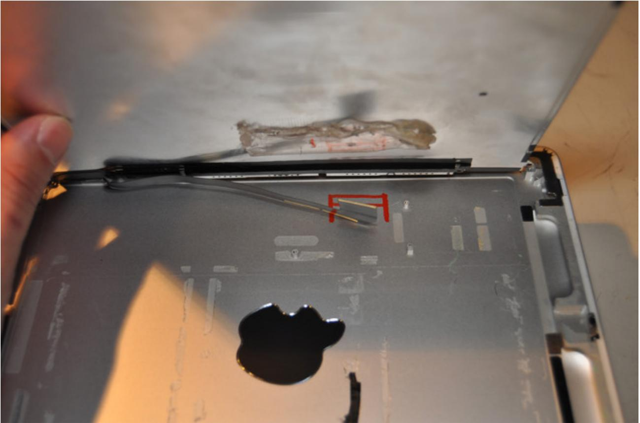
Once the cut is made, verify that your ribbon fits well, and is not flexed. (Ignore that second cut below the main one. It's not necessary.)
