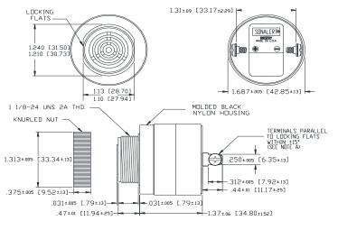
NOTE A: TERMINALS-.032 BRASS TIN PLATED, TAPPED FOR #6-32 SCREW. TWD #6-32 NICKEL PLATED BRASS SCREWS INCLUBED. WILL ACCEPT 1/4\* QUICK CONNECT.
