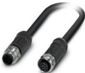
Sensor/Actuator cable, 8-position, PE-X/PE-X halogen-free, black-gray RAL 7021, shielded, Plug straight M12, A-coded, on Socket straight M12, A-coded, Cable length: 2 m, for outdoor applications, with high-grade steel knurl
