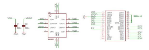
BMA255 shuttle board electrical layout
