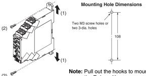
Note: Pull out the hooks to mount the Relay with screws.
