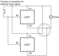
The power supply circuits for H3DT-series Timers use switching mode. Therefore, if there is a transformer or other device with a large inductance component on the power supply line, the inductance will cause a reverse voltage. If that occurs, insert a CR filter in the power supply line to reduce the reverse voltage.
