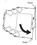
• To remove the Timer, insert a screwdriver into the hook on the top or bottom and pull out the hook to release the Timer.
