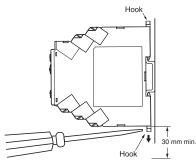
• It will be easier to mount and dismount the Timer if a distance of 30 mm or more is provided between the bottom of the Timer and other equipment.
