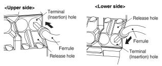
If a wire is difficult to connect because it is too thin, use a flat-blade screwdriver in the same way as when connecting stranded wire.
