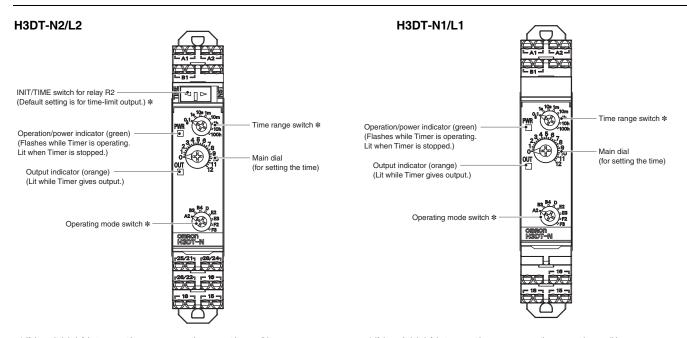
\* If the switch is left between settings, proper operation may not be possible. Make sure that the switch is set properly.
