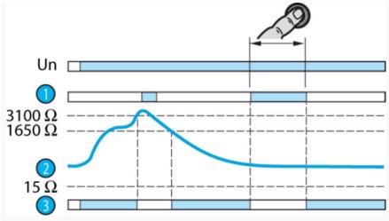
Version HWTM2 has a "test/reset" button for checking the operating state of the temperature control: When the temperature is normal, pressing the "test/reset" button simulates overheating, the yellow LED is extinguished and the contact of the "temperature" output relay opens; if "memory" mode is active, the fault indication is latched (the button must be released for at least 50 ms, then pressed again to reset the function).
