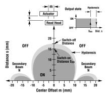
A minimum distance of s=3 mm must be maintained in the case of lateral approach in order to prevent entry into the operating range of the secondary beams.
