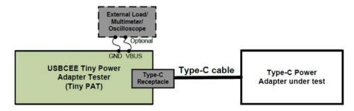
USBCEE Tiny PAT System Setup
