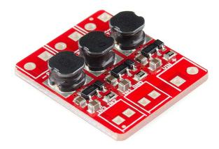
Developed in collaboration with Ethan Zonca of protofusion, the PicoBuck is a small-size triple-output constant current LED driver. By default, each channel is driven at 350mA; that current can be reduced by either presenting an analog voltage or a PWM signal to the board.
