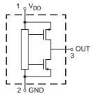
Fig. 1-1: Pin configuration
