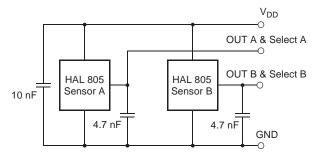
Fig. 4-2: Parallel operation of two HAL 805
