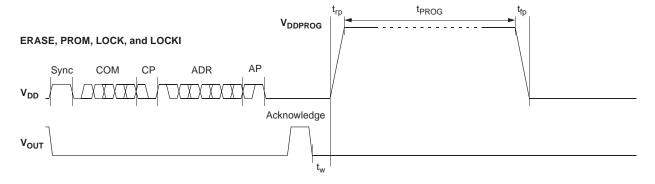
Fig. 5–4: Telegram for coding the EEPROM programming
