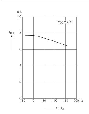
Fig. 3-3: Typical current consumption versus ambient temperature
