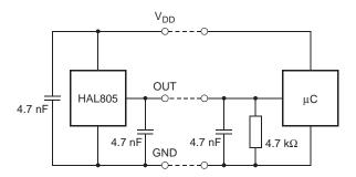
Fig. 4-1: Recommended application circuit
