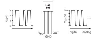
Fig. 2–1: Programming with V<sub>DD</sub> modulation
