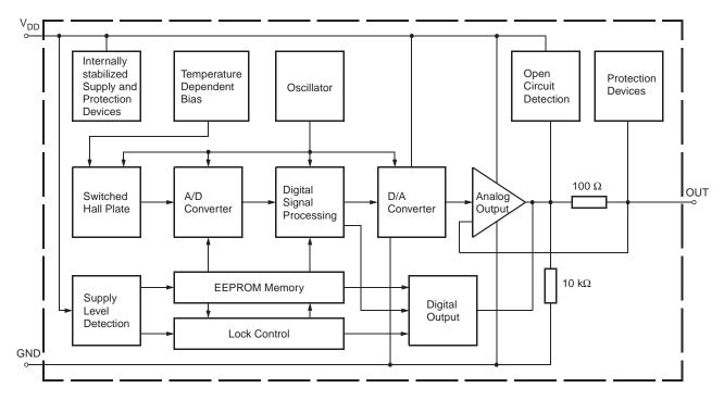
Fig. 2-2: HAL 805 block diagram
