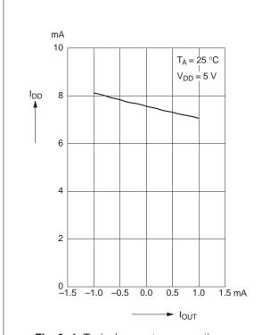
Fig. 3-4: Typical current consumption versus output current
