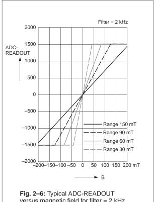
versus magnetic field for filter = 2 kHz
