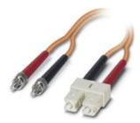
Assembled FO cable, zip cord cable, multi-mode fiberglass  $62.5/125 \, \mu m$ , OM1, plug: FSMA/SC duplex, degree of protection: IP20, for installation in cable ducts or control cabinets
