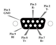
Termination is the 120  $\Omega$  resistor between T+ and T-.
