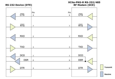
Figure 2-03. RS-232 DTE Device (male DB-9 connector) wired to a DCE RF modem (female DB-9)
