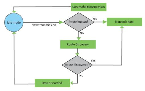
When DigiMesh data is transmitted from one node to another, the destination node transmits a network-level acknowledgment back across the established route to the source node. This acknowledgment packet indicates to the source node that the destination node received the data packet. If the source node does not receive a network acknowledgment, it retransmits the data. For more information, see Data transmission and routing.
