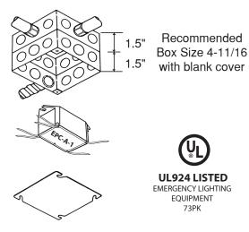
EPC-A-1 can also be mounted in plenum, when tiles are removable.
