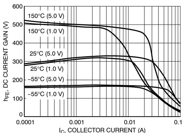
Figure 2. DC Current Gain vs. Collector Current
