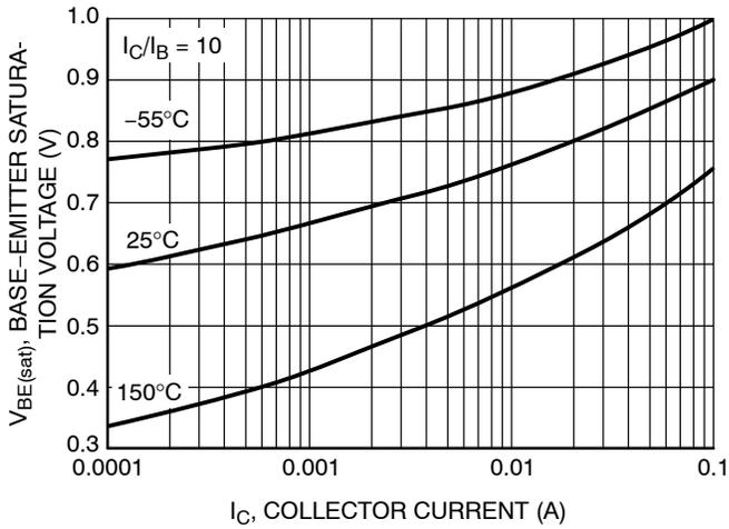
**Figure 3. Base Emitter Saturation Voltage vs. Collector Current**
