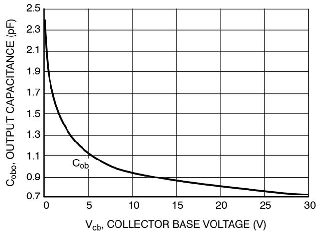
**Figure 7. Output Capacitance**
