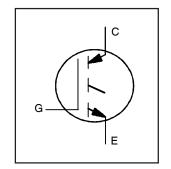
600 V  $I_{C(nom)} = 48A$ VCE(on) typ. = 1.65V @  $I_{C(nom)} @ 25^{\circ}C$ Motor Control IGBT
