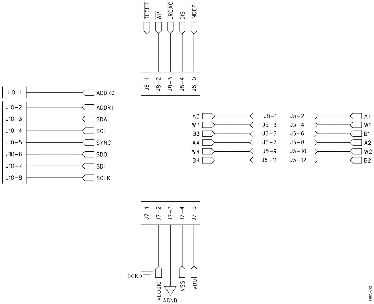
Figure 12. Schematic of Connectors to Daughter Board
