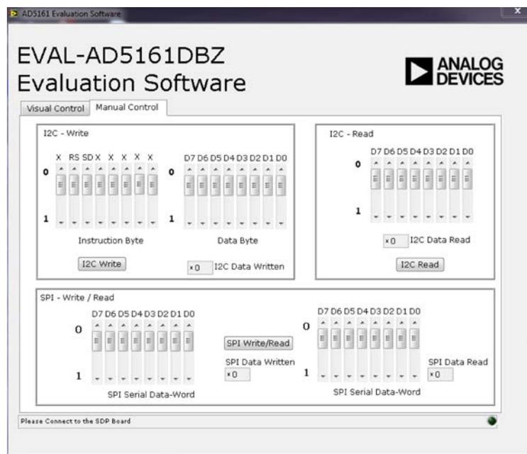
Figure 9. EVAL-AD5161DBZ Software Main Window, Manual Control Tab
