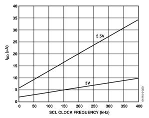
Figure 11. Standby Supply Current vs. Clock Frequency
