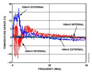
Figure 7. Temperature Error vs. Power Supply Noise Frequency
