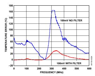
Figure 9. Temperature Error vs. 100 mV Differential Mode Noise Frequency (With and Without R-C-R Filter of 100  $\Omega$ –2.2 nF–100  $\Omega$ )
