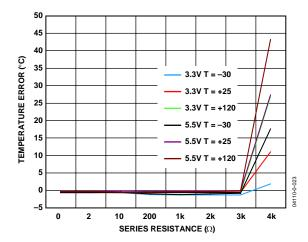
Figure 15. Temperature Error vs. Series Resistance
