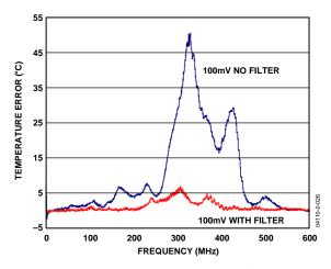
Figure 13. Temperature Error vs. 100 mV Common-Mode Noise Frequency (With and Without R-C-R Filter of 100  $\Omega$ –2.2 nF–100  $\Omega$ )
