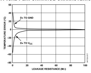
Figure 4. Temperature Error vs. Leakage Resistance
