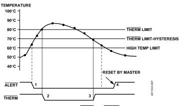
Figure 21. Operation of the ALERT and THERM Interrupts
