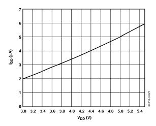
Figure 12. Standby Current vs. Supply Voltage
