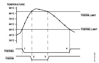
Figure 22. Operation of the THERM and THERM2 Interrupts
