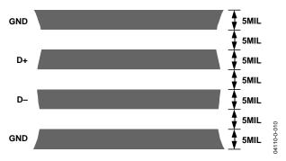
Figure 24. Typical Arrangement of Signal Tracks
