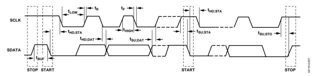
Figure 2. Serial Bus Timing
