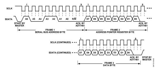
Figure 17. Writing a Register Address to the Address Pointer Register, then Writing Data to the Selected Register
