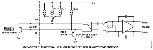
Figure 16. Input Signal Conditioning
