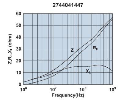
Impedance, reactance, and resistance vs. frequency.
