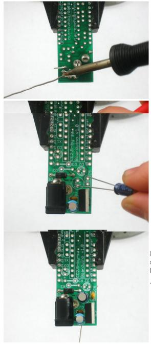
Now you should soder in the 6.3V electrolytic capacitor **C4** as shown. Remember its polarized so you must place the longer lead in the positive-marked hole.
