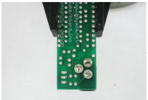
Make sure all three pads are soldered, with plenty of solder, the holes should be filled up. This gives the jack mechanical strength.
