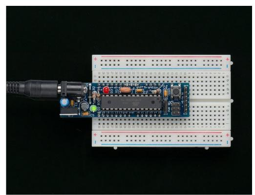
If you've ever struggled to use a solderless breadboard with an Arduino, you understand how frustrating it can be! I designed this Arduino clone to solve this problem in an inexpensive DIY fashion. <u>Kits with all parts are available in the Adafruit webshop</u> (http://adafru.it/aJD).
