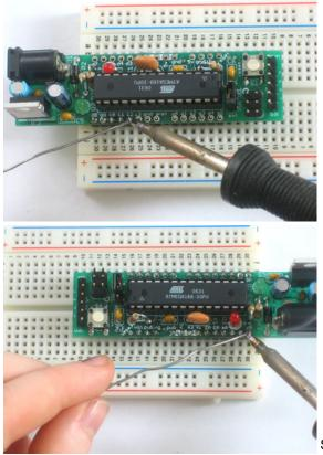
Solder all of the pins of the header, making sure that the board is sitting flat against the header.
