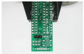
Place the 3 pin header at the other end of the board as shown. the short end goes into the PCB, and the long ends extend up.
