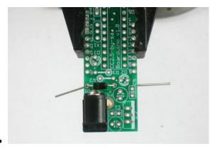
Next, place the 1N4001 diode  $\mathbf{D1}$ . Diodes are directional, they only let current flow in one direction. This diode is used to protect the Boarduino from damage. Make sure the white stripe on the diode matches the white stripe in the silkscreened image below. In this picture, the stripe is on the right.
