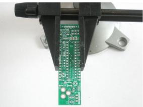
Place the PCB in a vise to make soldering easy! Heat up the soldering iron to 700 degrees, tin it if necessary. Make sure the sponge is wetted.
