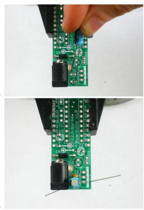
Next, its time to place the 25V electrolytic capacitor**C3**. Electrolytic capacitors are *polarized* which means they only work well in one direction. Put it in backwards and they can explode! You can tell how to place it because the silkscreened image has a plus near one hole and the capacitor has one long lead. That lead is the positive lead. In this image, its the one on the right.
