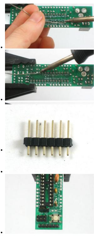
Solder in the socket by tacking two opposite corners and then soldering the rest of the pins. Press the socket into the board to make sure its flat up against it.
