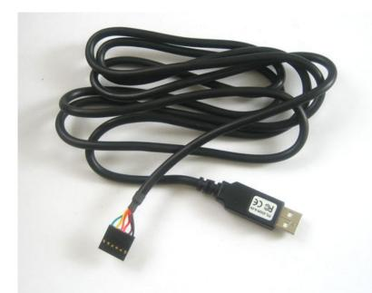
The easiest way to start loading Arduino sketches into the DC Boarduino is to use a FTDI USB cable. These cables have the USB chip *inside the cable* and a 6-pin socket on the end.
