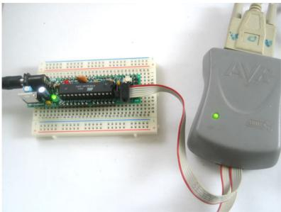
There is also a standard 6-pin ICSP (In-Circuit Serial Programming) cable that can be used to burn a new bootloader or just reprogram the chip.
