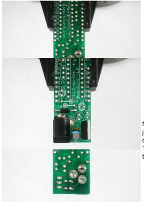
Next is the 5V regulator. This takes the power from the DC jack which may be something like a 9V battery, and brings it down to 5V, which is suitable for the microcontroller chip. This part must be placed as shown, with the metal heat sink tab on the right.
