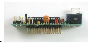
Carefully remove the boarduino by slowly rocking it back and forth to release it from the solderless breadboard.
