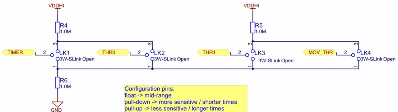
Figure 7.2 Minimal resistor strap configuration
