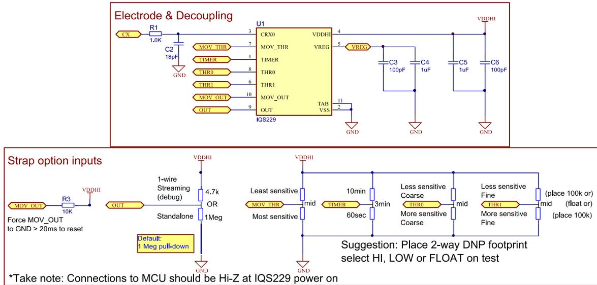
Figure 3.1 Reference schematic
