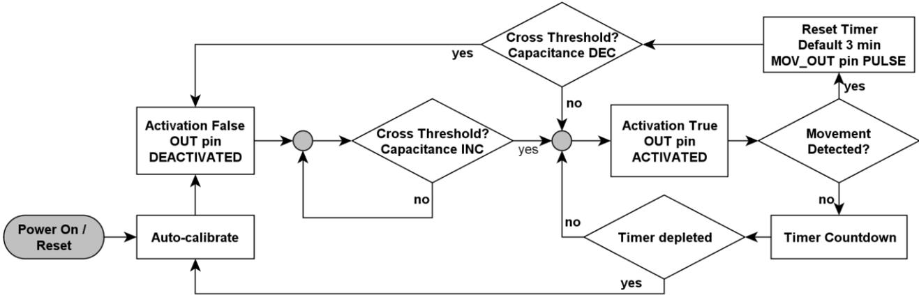
Figure 1.1 Flow diagram of the IQS229 user interface
