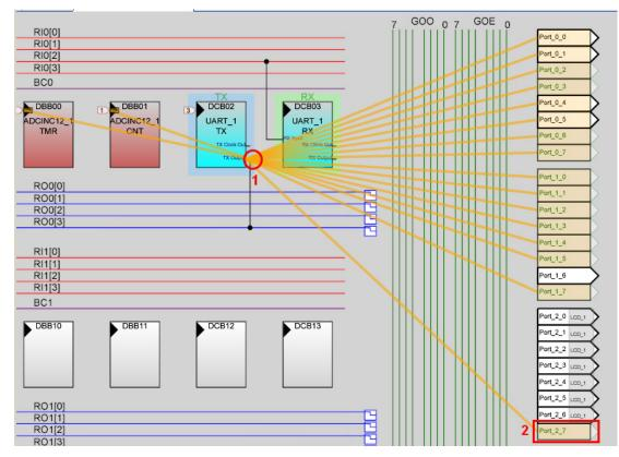
b. Manual Routing: Configure the LUT on Row\_0\_Output3. To do so, click on **Row\_0\_Output3** to open the Digital Interconnect window.
