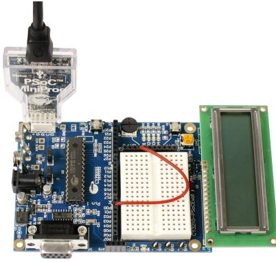
The board can be programmed either through PSoC Designer IDE or by launching PSoC Programmer. To program the board using PSoC Programmer, see Programming Specifications and Connections on page 20. To program the board through PSoC Designer, follow these steps. **Note** When programming the board through PSoC Designer, close any open instance of PSoC Programmer.
