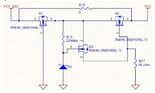
Figure 4-4. Protection Circuit
