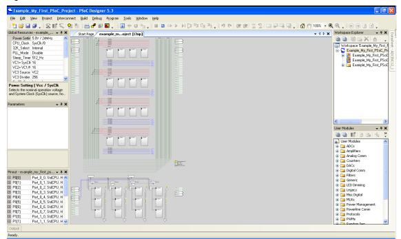
9. Configure the modules required for this design. Also, connect the modules together and to the pins on the PSoC. In the User Modules section, expand the **ADCs** folder.
