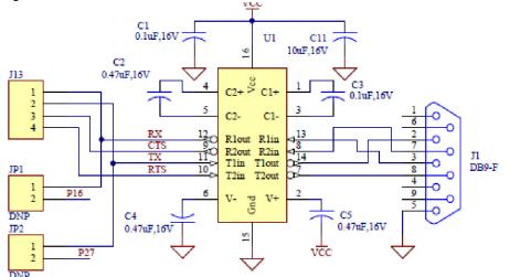
Figure 4-7. RS-232 Interface Schematic
