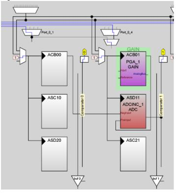
Figure 5-10. PGA User Module Placement
