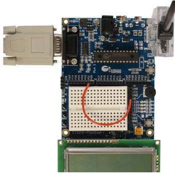
Figure 5-32. CY3210-PSoCEVAL1 Connected to RS-232 Cable
