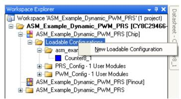
The new configuration can be renamed based on the project. All PSoC resources (digital and analog blocks) can be reused. A loadable configuration can be deleted if no longer required. However, the base configuration (the default configuration) cannot be deleted.
