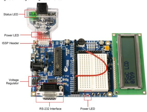
Figure 3-2. Programming PSoC Device
