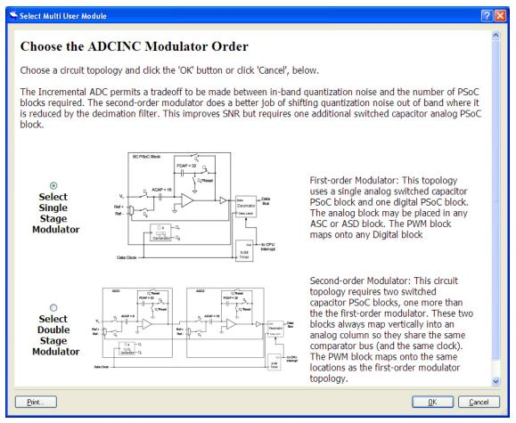
The user module (UM) is placed in the first available analog block. By default, the UM is placed on an Analog Switched Capacitor Type C block. It should be shifted to a Switched Capacitor Type D block, as explained in the next step.
