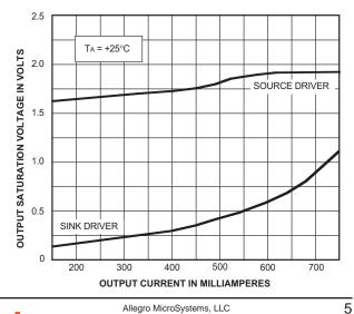
Typical output saturation voltages showing Satlington sink-driver operation.
