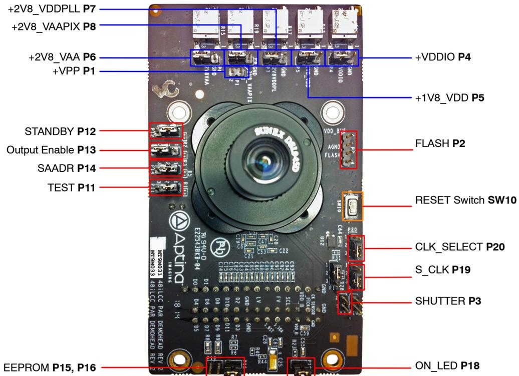
Figure 3. Top View of Evaluation Board – Default Jumpers
