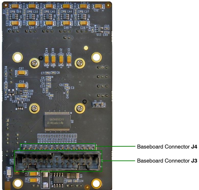
Figure 4. Bottom View of the Evaluation Board – Connector
