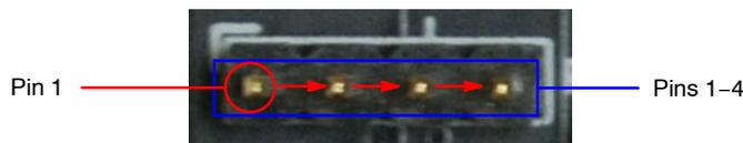
**Figure 5. Pin Locations for a Single Jumper.**
