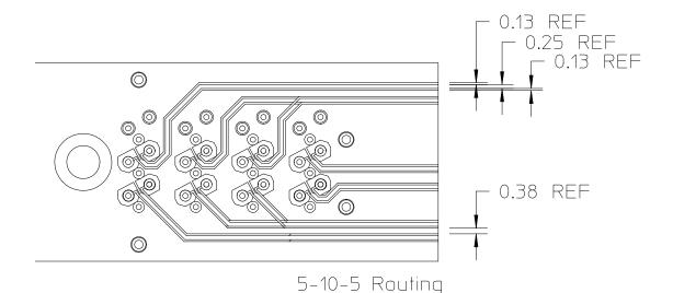
Showing 3 layer overlaid for a single connector (2 signal and ground layer)
