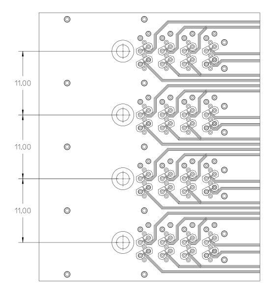
Showing 3 layers overlaid for a typical side by side stacking (2 signal and ground layer)
