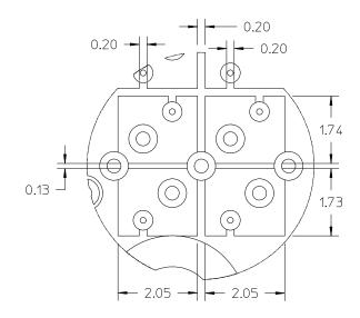
Chamfers may be eliminated, but must be done in a balanced fashion Signal and Non-Signal features may be mixed on a layer
