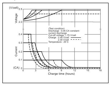
In order to fully utilize the characteristics of VRLA batteries, constant-voltage charging is recommended. For details of charging see page 19.
