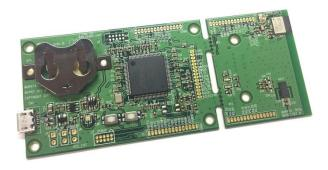
The MBN52832 Development Kit is designed to facilitate application development using the Nordic nRF52 SDK. The EVB supports the same J-Link USB-SWD and USB-UART interfaces as those provided by the nRF52 DK to ease the debugging and development process.
