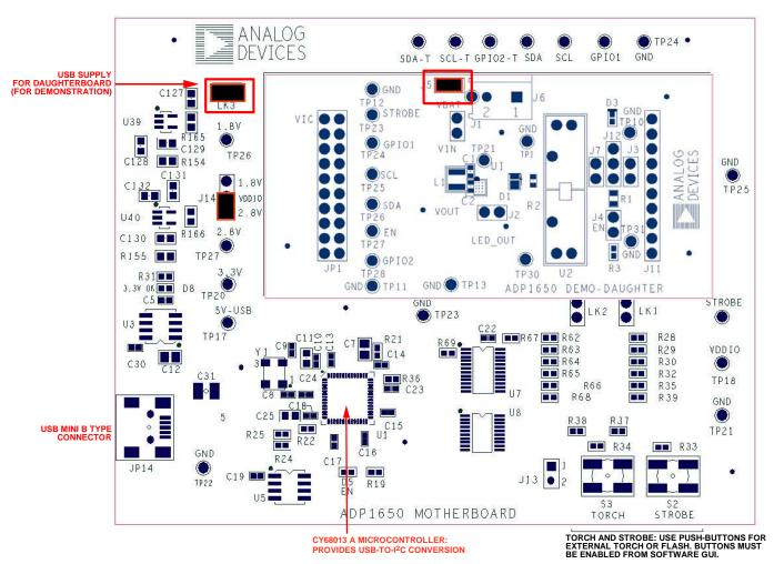
Figure 11. Powering the ADP1650 from a USB Port
