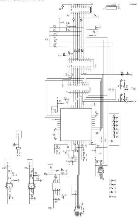
Figure 12. ADP1650 Evaluation Motherboard Schematic
