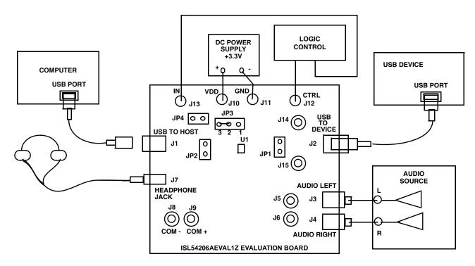
FIGURE 2. BASIC EVALUATION TEST SETUP BLOCK DIAGRAM
