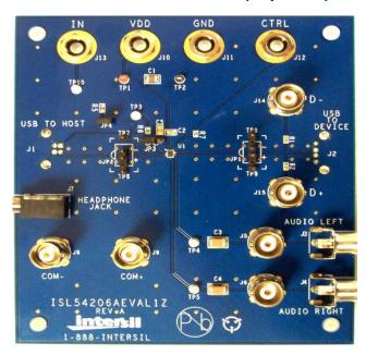
FIGURE 1. ISL54206AEVAL1Z EVALUATION BOARD
