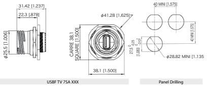
Jam nut receptacle Hexagonal Nut mounting: Shell type 7
