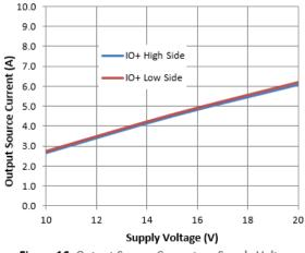
Figure 16. Output Source Current vs. Supply Voltage
