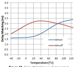
Figure 15. Delay Matching vs. Temperature
