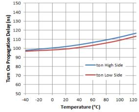
Figure 5. Turn-on Propagation Delay vs. Temperature
