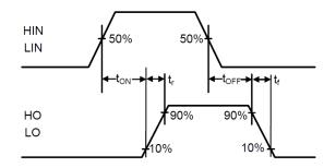
Figure 2. Switching Time Waveform Definitions
