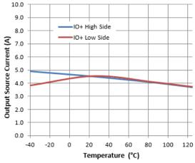
Figure 17. Output Source Current vs. Temperature
