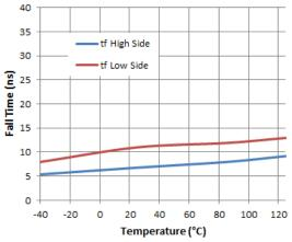
Figure 11. Fall Time vs. Temperature
