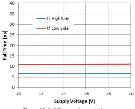
Figure 10. Fall Time vs. Supply Voltage
