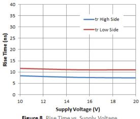
Figure 8. Rise Time vs. Supply Voltage
