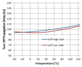
Figure 7. Turn-off Propagation Delay vs. Temperature
