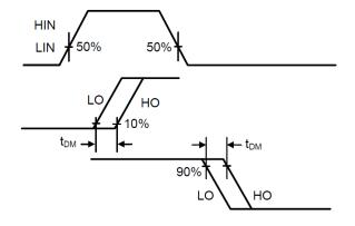
Figure 3. Delay Matching Waveform Definitions
