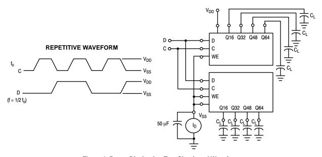
Figure 1. Power Dissipation Test Circuit and Waveform
