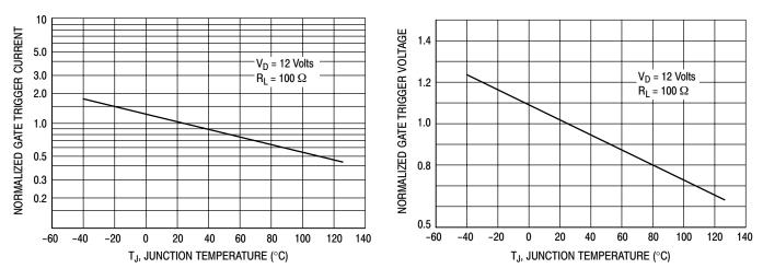
Figure 6. Gate Trigger Current
