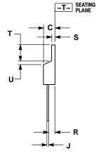
NOTES: 1. DIMENSIONING AND TOLERANCING PER ANSI Y14.5M, 1982. 2. CONTROLLING DIMENSION: INCH.
