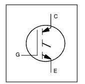
600 V  $I_{C(nom)} = 10A$ VCE(on) typ. = 1.6V @  $I_{C(nom)} @ 25^{\circ}C$ Motor Control IGBT
