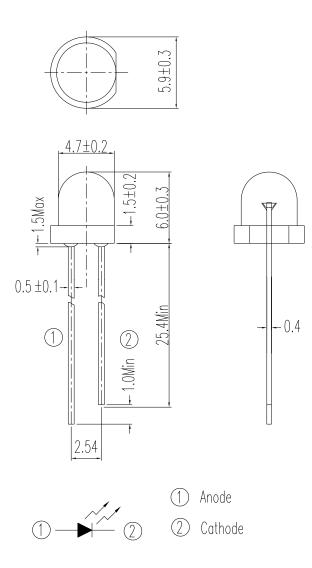
Note: Tolerances unless dimensions ±0.25mm
