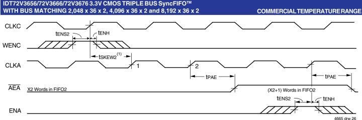
1. tskew2 is the minimum time between a rising CLKC edge and a rising CLKA edge for AEA to transition HIGH in the next CLKA cycle. If the time between the rising CLKC edge and rising CLKA edge is less than tskew2, then AEA may transition HIGH one CLKA cycle later than shown.
