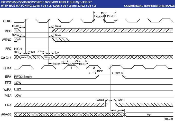
1. tskew1 is the minimum time between a rising CLKC edge and a rising CLKA edge for EFA to transition HIGH in the next CLKA cycle. If the time between the rising CLKC edge and rising CLKA edge is less than tskew1, then the transition of EFA HIGH may occur one CLKA cycle later than shown.
