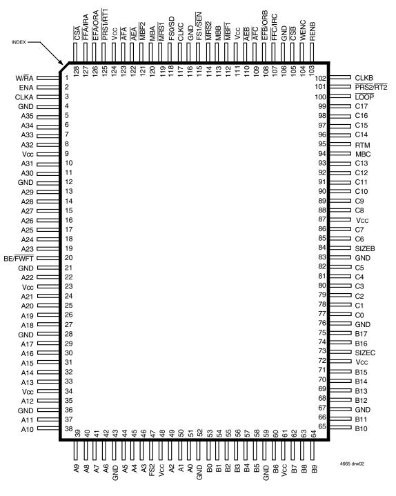
TQFP (PK128-1, order code: PF) TOP VIEW each port are independent of one another and can be asynchronous or coincident. The enables for each port are arranged to provide a simple bidirectional interface between microprocessors and/or buses with synchronous control.
