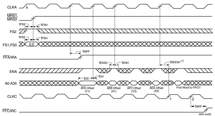
1. tskewi is the minimum time between the rising CLKA edge and a rising CLKC edge for FFC/IRC to transition HIGH in the next cycle. If the time between the rising edge of CLKA and rising edge of CLKC is less than tskewi, then FFC/IRC may transition HIGH one CLKC cycle later than shown.
