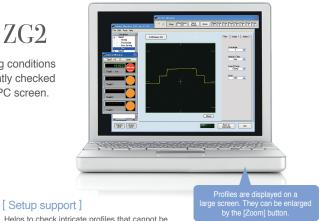
Helps to check intricate profiles that cannot be sufficiently checked on the controller's LCD monitor and provides easy-to-view setting lists for easy setting.
